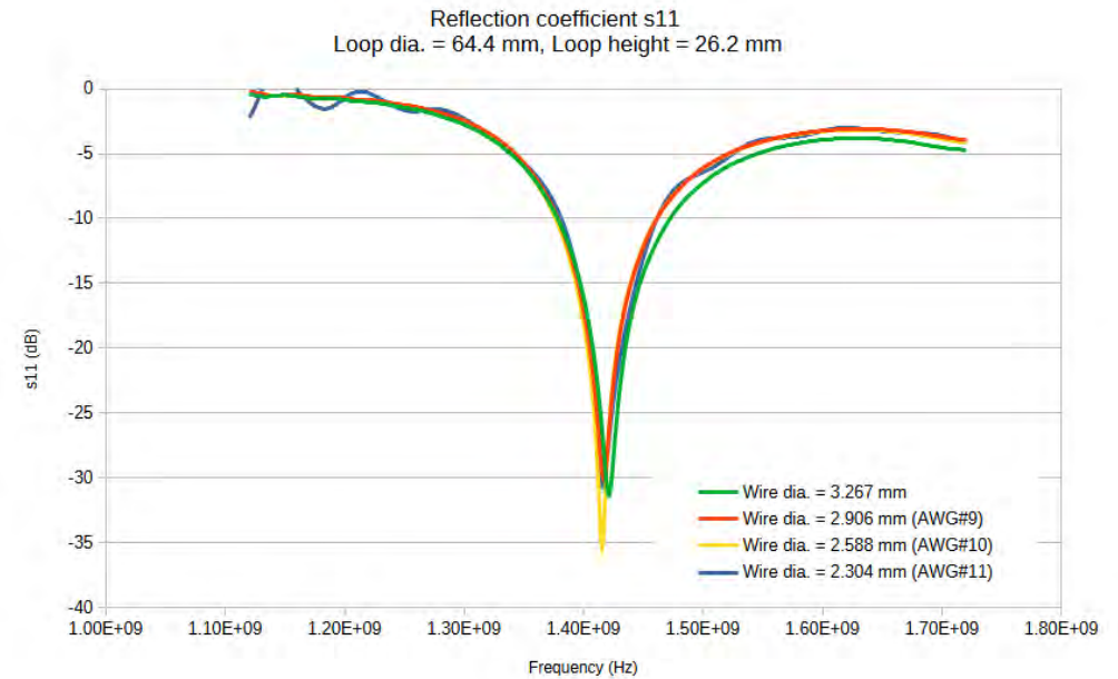
Figure – 7 : Changes in s11 characteristics
