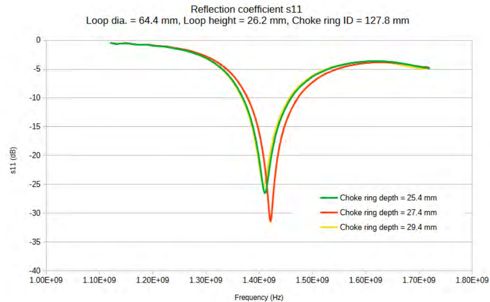
Figure – 11 : Changes in s11 characteristics
