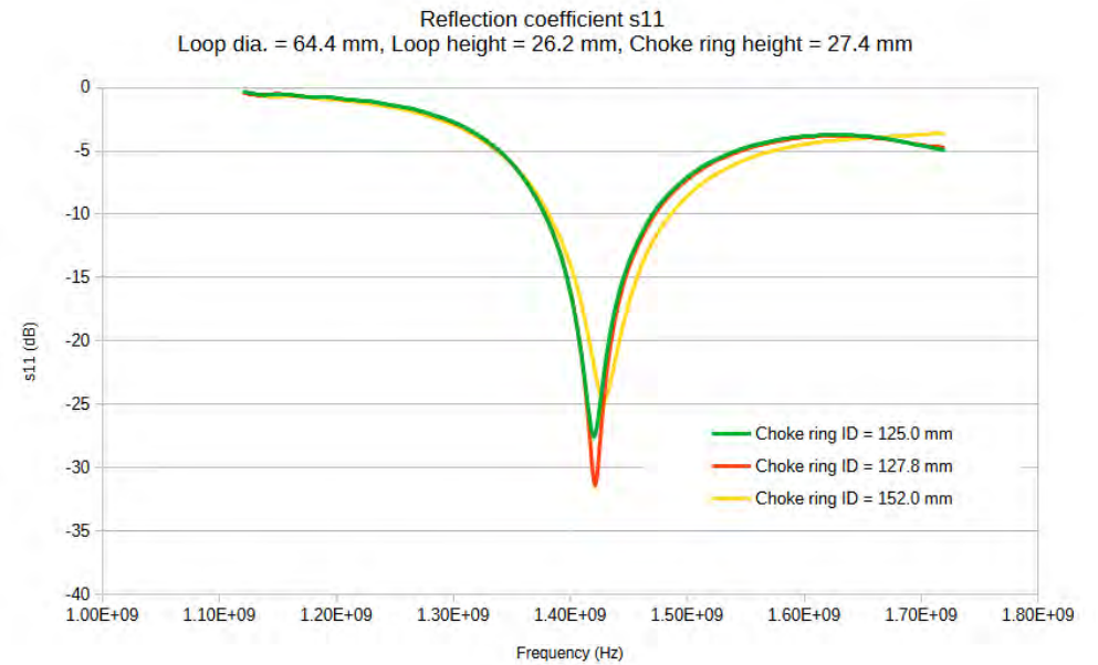
Figure – 9 : Changes in s11 characteristics
